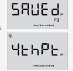
11. Press the **Cal** key to save and end the calibration. The **Cal** key can be pressed when either the "SAVEd" or "4thPt" screens is shown.
